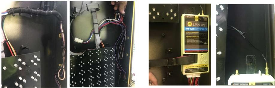
4. Unscrew +Ve wire on 4 way connector pin 1 and crimp to +Ve crimp connector of new wire harness
