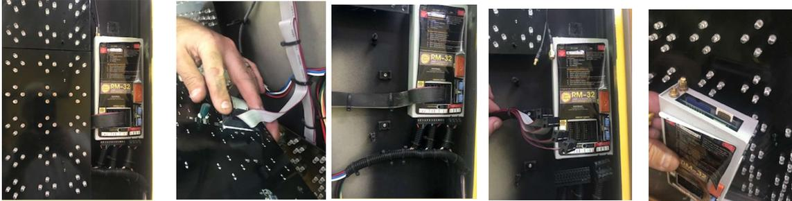
3. If fitted Remove small battery inside sign head below controller, disconnect wires. Proceed to remove the cable covering (if fitted) to expose the wires. Fit the New Controller (with the wiring harness fitted) into the sign and plug the 4 Ribbon Cables back in. Plug the original aerial wire into the right side as shown. Cut of the small GPS cable and tie to the cable as shown.
