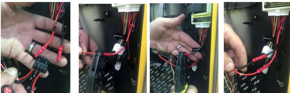
5. Unscrew Fan -Ve wire from 14 way connector pin 2 and crimp to -Ve Fan connector of new wire harness. (the Negative wire is the one with the stripe on the actual wire)
